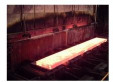
Hot Steel Slab Exiting the Furnace
